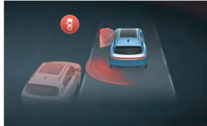
When the Door opening warning (DOW) detects moving objects such as pedestrians and moving vehicles in the area behind the vehicle through radar, and the speed of the subject vehicle is lower than 3 km/h, the vehicle will send out a warning message when the occupants open the door to remind them to pay attention to the current situation.
