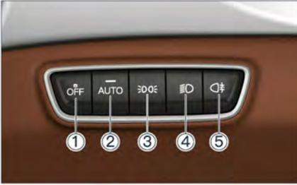
The light combination switch is located on the left side of the instrument panel.
