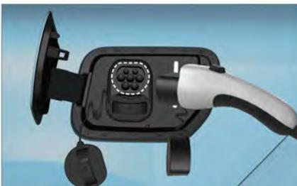
3. According to the prompt of the charging pile interface, start the charging process;
