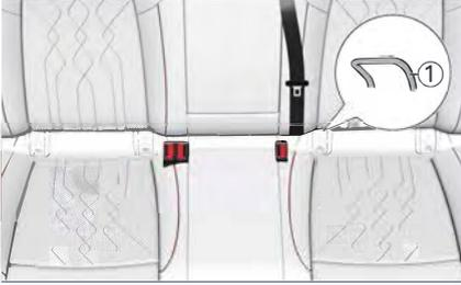
1. Place the child safety seat on the seat, find the lower fixing point ① , and insert the lower mounting slot (as indicated by the arrow in the above figure) of the child safety seat into the lower fixing point ① in the gap of the seat cushion until an engagement sound is heard;
