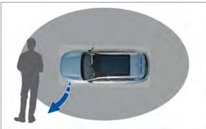
After the START/STOP button is turned off, you can close all the doors and the POT, and keep away from the vehicle with the smart key to allow the doors to be locked automatically. At this time, the left and right turn signal lamps will flash once, the horn will sound once, the exterior mirrors will fold automatically, and the hidden door handles will retract automatically.
