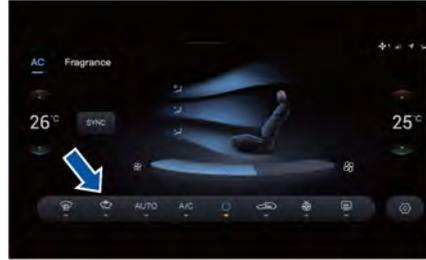
On the A/C interface of the CSD, click the deicing/snow removal icon to turn on the front windshield deicing/snow removal function. The system will adjust:
