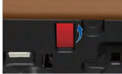
Pull the engine hood opening handle twice in a row and lift the engine hood to open it. After the engine hood is opened, the above message will appear in the instrument cluster.
