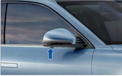
The left and right cameras are located at the outer bottom of the left and right rearview mirrors, and are used to record the side area of the vehicle.
