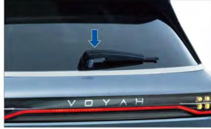
1. Lift the rear wiper arm and wipe off the dust and dirt on the rear wiper blade with a soft cloth;
