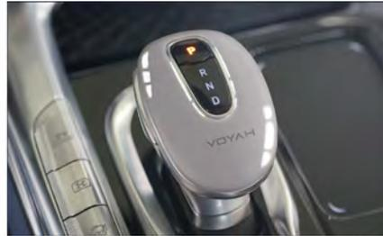
The vehicle has four gears: P, R, N, and D. After the vehicle enters the READY state, depress the brake pedal and switch gears, the corresponding gear light on the shift handle will light up, and the corresponding gear will be displayed on the instrument cluster.
