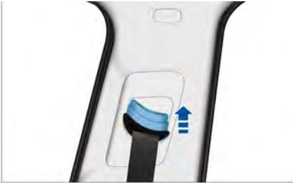
**Move down:** Press the release button of the height adjuster and move it downward (in the direction indicated by the arrow in the figure below), adjust the shoulder belt to an appropriate height as needed, and then release the release button. When you hear a "click" sound, it means the adjuster is locked.
