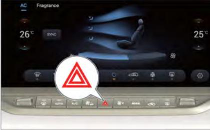
The hazard warning lamp switch is located in the middle of the A/C control panel.
