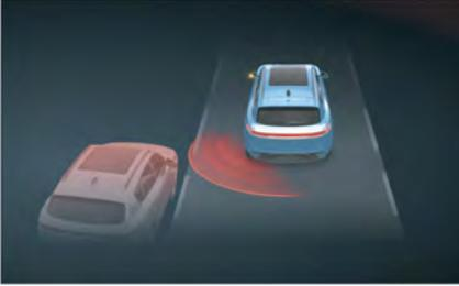
BSD/LCA mainly monitor the adjacent lanes behind the vehicle through radar sensors, remind drivers to pay attention to driving safety in time, and give prompts when changing lanes.
