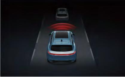
The FCW monitors the risk of collision between the subject vehicle and objects such as pedestrians and vehicles ahead through MMW radar and smart front-view camera. When there is a risk of collision, the vehicle will emit an audible and visual alarm to alert the driver.
