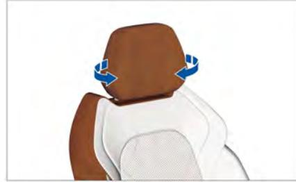
Adjust the wings on both sides inward and outward.
