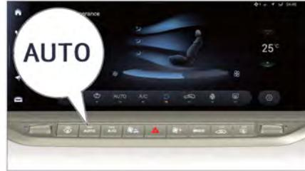
Press the auto mode button, the button indicator will go up, the A/C system will enter the automatic mode, and the following items will be automatically controlled according to the set temperature value:
