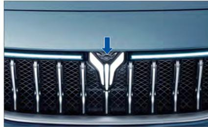
The front view camera is located above the front bumper logo and is used to record the area in front of the vehicle.
