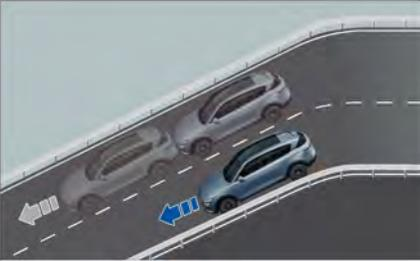
Hill descent control (HDC) can be used to actively brake and decelerate when the vehicle is passing through a steep downhill section, so that the vehicle can move safely and smoothly.
