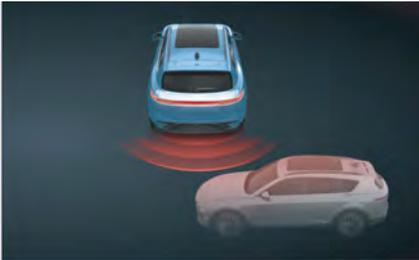
When the vehicle shifts into the R gear (reversing), the RCTA detects through the radar that there are pedestrians, moving vehicles or moving objects approaching on the left and right sides of the rear of the vehicle, and there is a risk of collision, the CSD will prompt an alarm message, accompanied by a warning sound, to remind the driver to avoid safety accidents.
