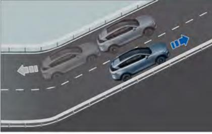
Hill start assist (HSA) can prevent the running vehicle from slipping backward when starting uphill, or sliding forward when reversing downhill. During this process, the driver does not need to operate the EPB button, thus effectively reducing the difficulty of starting or reversing on the slope.
