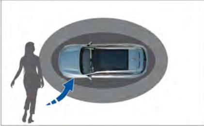
When you approach the vehicle with the smart key, the door will automatically unlock, the left and right turn signal lamps will flash twice, and the exterior rearview mirrors and concealed door handles will automatically deploy.
