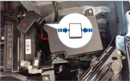
1. Open the engine hood and remove the engine compartment trim panel;
