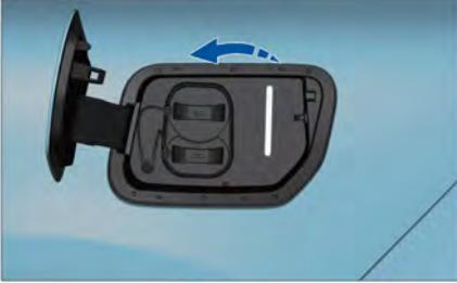
Swipe right on CSD interface to show the -1 screen, touch the Open C. Port, and the charging cover will automatically pop open. After the charging cover is opened, you can manually press it inward to close it.
