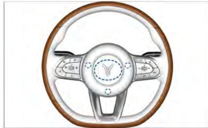
Press the position within the dotted area of the steering wheel in the figure above, the horn will sound, and release it to stop the sound.
