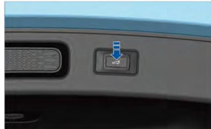
Press the POT inner closing switch
