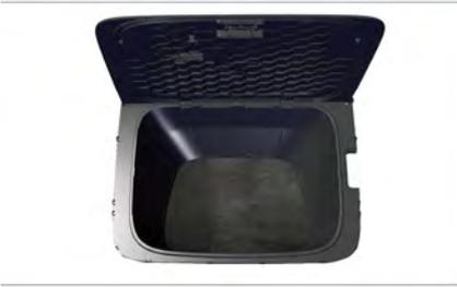
The front trunk (for EV) is located in the engine compartment. Open the engine hood and pull the front trunk release handle to open the front trunk, which can be used for loading items.
