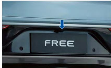
The rear view camera is located next to the license plate lamp in the rear bumper and is used to record the area behind the vehicle. When R gear is engaged, and the reversing dynamic assist line will be shown on the display.
