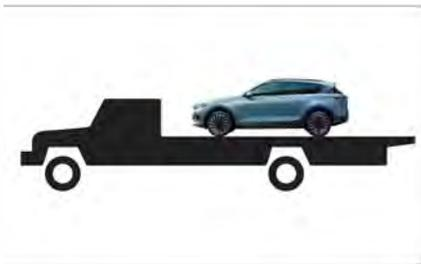
As the best way to transport the vehicle, it loads and transports the vehicle directly on the truck.
