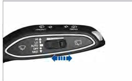
When the wiper stalk is in the AUTO position, turn the knob to the left to increase the auto wiper sensitivity; turn the knob to the right to reduce the auto wiper sensitivity.
