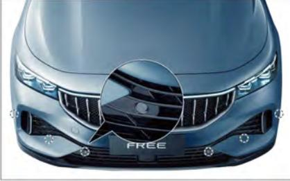
The front PDC is mounted on the front bumper of the vehicle.(6 in total).
