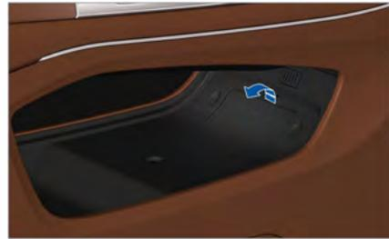
3. Remove the new fragrance protective film, put in the new fragrance, and refit the fragrance plug and storage box pad.
