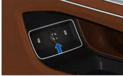
The front 12V power interface is located under the central armrest and can be used when the trim cover is opened. The maximum allowable power is 120W.
