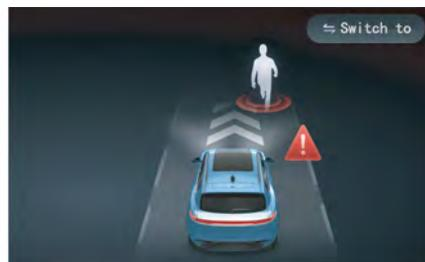
The NVS provides clear images at night and displays detailed information of the road, such as pedestrians, vehicles, lane markings, traffic signals, etc., thereby providing drivers with more comprehensive and accurate road information and issuing hazard warnings in advance.
