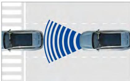
Front vehicle start reminder (FVSR) is a driving safety assistance function, and the following conditions must be met to trigger the FVSR function:
