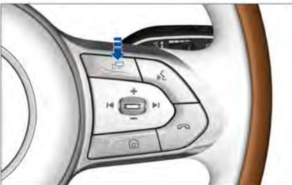
The display information of the instrument cluster can be switched by the menu button
