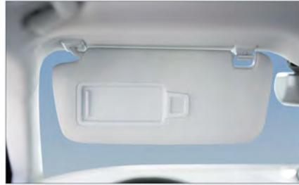
Rotate the sun visor down to block sunlight from the front.
