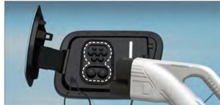
3. According to the prompt of the charging pile interface, start the charging process;
