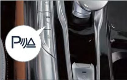
The front PDC is turned on by default after the vehicle is started. You can turn on/off the PDC through the PDC switch beside the shift lever.
