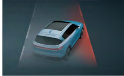
Lane keeping assist includes three safe driving assist functions: Lane departure warning (LDW), Lane keeping assist & departure warning (LKA) and Lane centering control (LCC).
