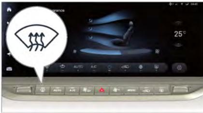
Press the front windshield defogging button, the button indicator will go on, the front windshield defogging function will be activated, and the system will automatically perform the following settings:
