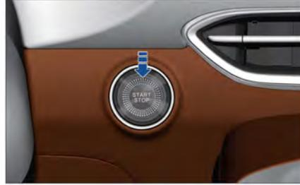
The vehicle is equipped with a START/STOP button. The START/STOP button can only be operated when the vehicle detects the smart key.
