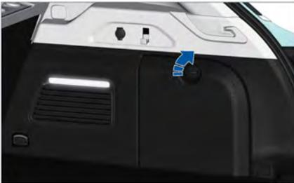
Turn the cover plate knob 90° clockwise to open the tool box cover plate, or turn it 90° counterclockwise to close the tool box cover plate.
