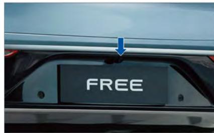
The rear license plate lamp is installed next to the rear view camera to illuminate the vehicle license plate.
