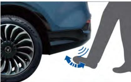
Approach the vehicle identification area with the smart key, then kick your toes into the middle of the rear bumper at least 10 cm, and the POT can be opened/closed.
