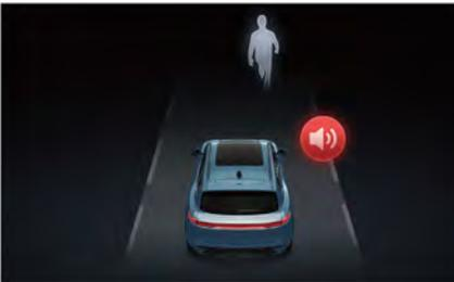
When the vehicle is running at a low speed, the low-speed pedestrian warning system will issue a warning sound for pedestrians approaching the vehicle to warn pedestrians to pay attention to safety.
