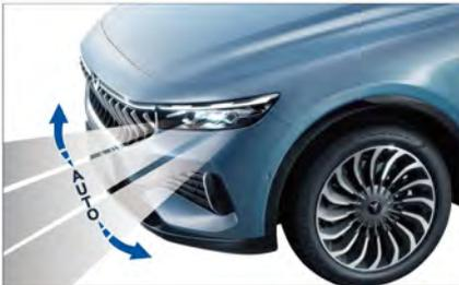
The AFS automatically adjusts the illumination angle of the headlamp according to the load status of the vehicle
