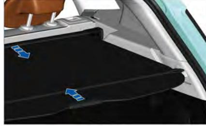
Unfolding: pull the curtain handle backward to fix the curtain in the grooves on both sides of the body.
