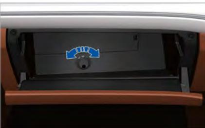
The glove box air outlet switch is located in the glove box.
