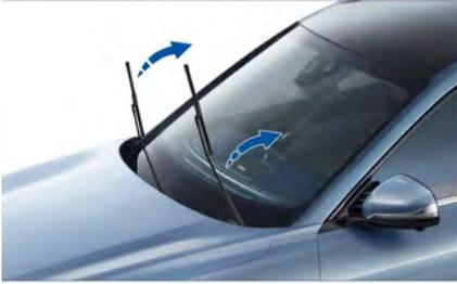
1. Enable front wiper maintenance mode, then the front wiper will stay on the left side of the front windshield;
