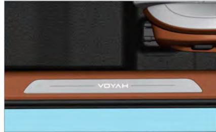
Side step welcome lamp is located on the door sill to provide illumination for occupants when getting on and off the vehicle.
