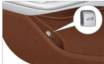
When the vehicle is stationary, lift up the driver side POT switch
