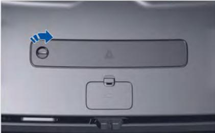
The warning triangle is stored on the POT inner trim panel. Open the POT, turn the cover plate knob clockwise along the arrow direction as shown in the above figure, open the cover plate, and take out the warning triangle.
