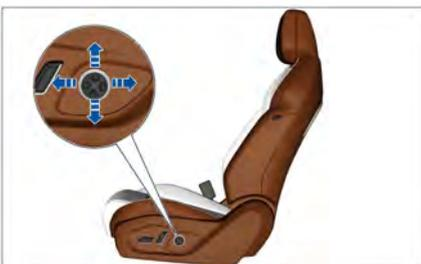
The lumbar support can be adjusted up, down, forward and backward by the adjustment button.
