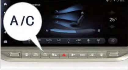
Press the A/C cooling button, the button indicator will go on, and the A/C system will activate the cooling function.
