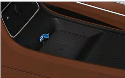
2. Remove the fragrance plug at the rear of the console (as shown by the arrow in the figure below), and take out the original fragrance;
