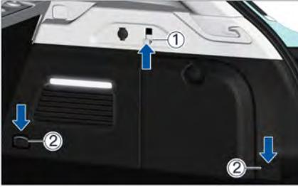
Hooks ① on the left and right sides of the trunk can be used for lighter items. Fixing rings ② on the left and right sides of the trunk can be used to bundle and fix larger items placed in the trunk.
