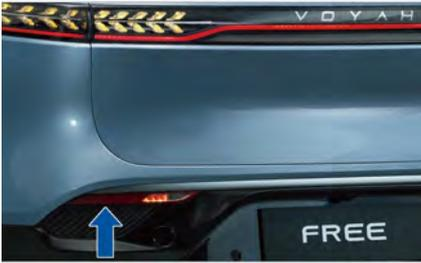
The rear retro-reflecting device is used to reflect the light from the vehicle behind, reminding the driver of the vehicle behind to keep a safe driving distance.
