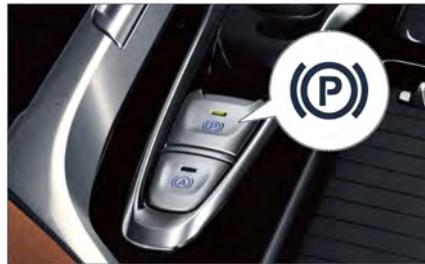
Activation: After the vehicle is stopped, lift up the EPB button / press the P gear button, the EPB indicator and button indicator on the instrument cluster will light up, and EPB will be activated.
