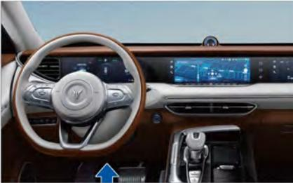
Footwell lamps are installed in front of the driver and the front passenger to provide illumination for the front row personnel when getting on and off the vehicle.
