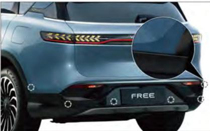
The rear PDC is mounted on the rear bumper of the vehicle.(6 in total).
