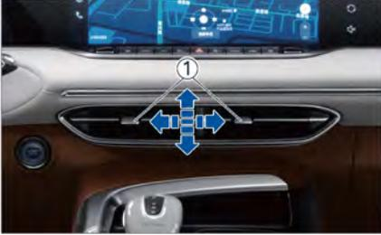
Move the grille up, down, left and right to adjust the air outlet direction, and move it to the left/right end to close the air outlet.
