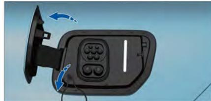
2. Connect the charging plug that comes with the charging pile to the DC charging port of the vehicle;
