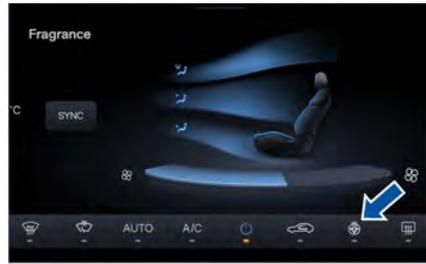
The steering wheel of this vehicle has heating function, which can be activated as needed to improve driving comfort. On the main interface of the CSD **>>** to enter the A/C interface, then click the steering wheel heating icon to heat the steering wheel.
