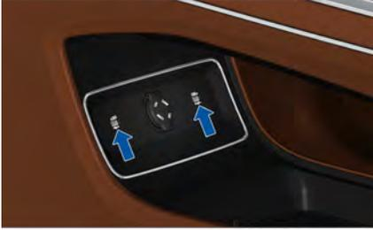
There are two USB Type-A interfaces under the front central armrest with the charging power of 10.5 W, which supports data transmission.
